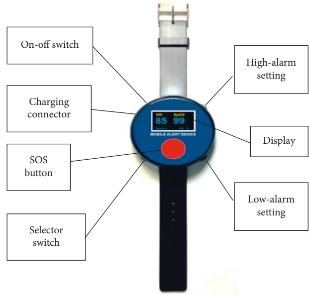
FIGURE 1: The signal sending part of the emergency alert device.
