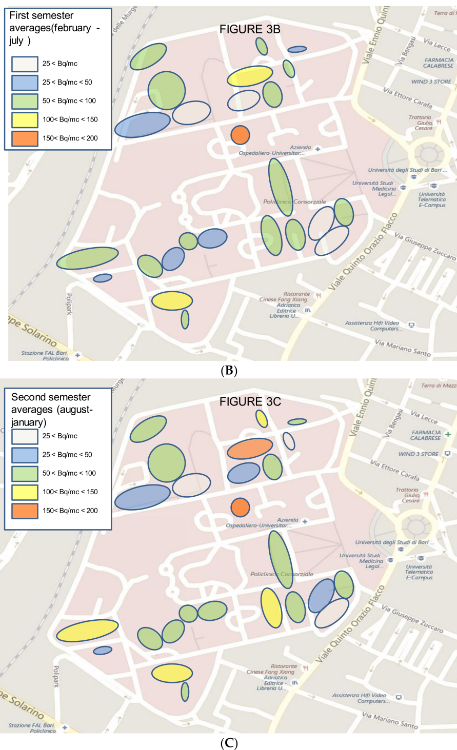
Figure 3. (A–C) Distributions of the radon concentrations in the different areas of the hospital as annual average and in the two periods, expressed as Bq/m 3 (scale 1: 100).
