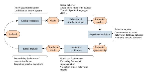
Figure 7. Basic simulation lifecycle.
