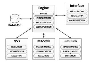
Figure 11. CPSS simulator architecture.
