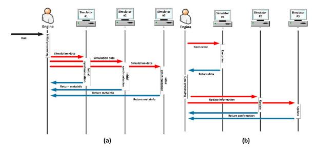
**Figure 8.** (a) Sequence diagram describing the initial synchronization process in a co-simulator; (b) Example of a sequence diagram about the stop-and-wait coordination mechanism when using a federated co-simulation controlled by a third-party engine.
