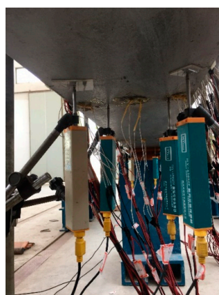
Figure 4. The arrangement of the displacement sensor.
