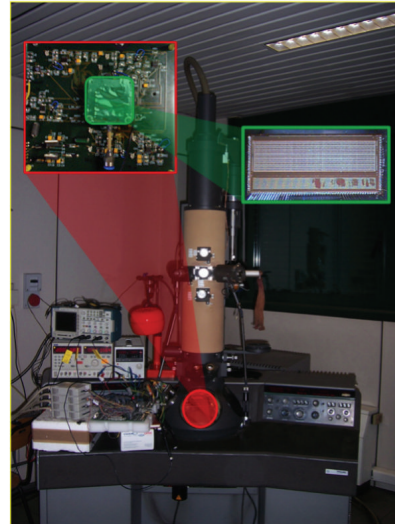
FIGURE 31: The transmission electron microscope (TEM), board and chip used in the experiment.
