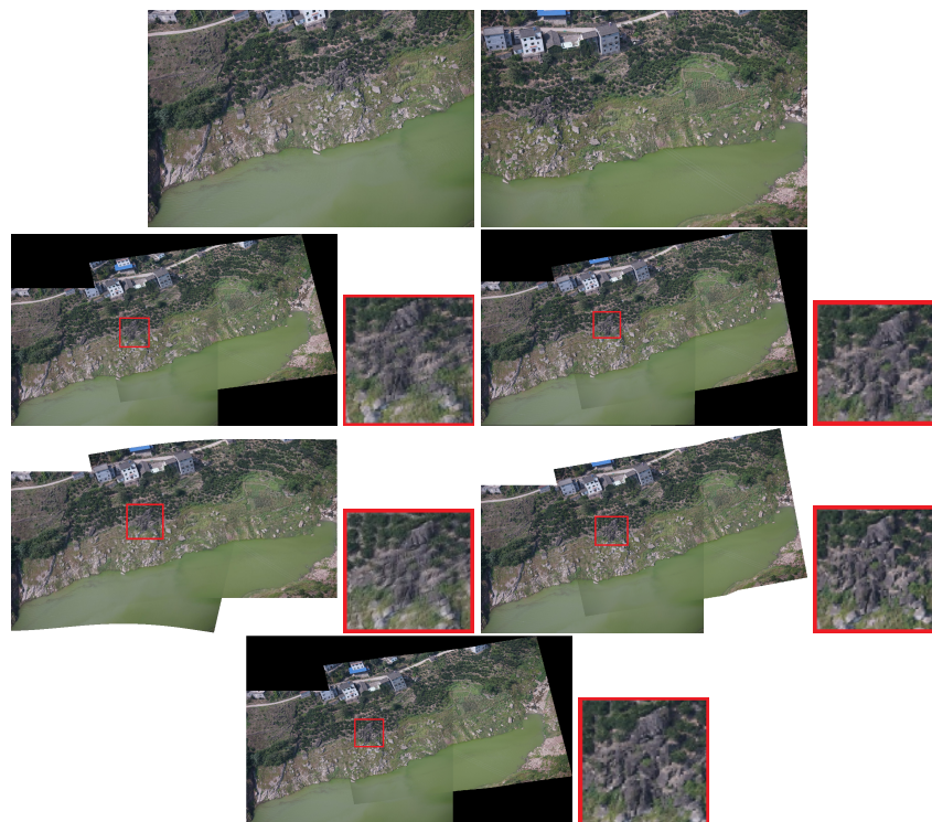
Figure 4. Qualitative comparison on UAV image mosaic. The first row is the two images to be stitched. The second and third rows are the stitching results of Autostitch [4], AANAP [41], SPHP [40], and PT [54]. Our result is shown in the last row. Red boxes highlight the ghostly parts.
