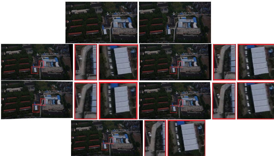
Figure 6. Qualitative comparison on UAV image mosaic. The first row is the two images to be stitched. The second and third rows are the stitching results of Autostitch [4], AANAP [41], SPHP [40], and PT [54]. Our result is shown in the last row. Red boxes highlight the ghostly parts.
