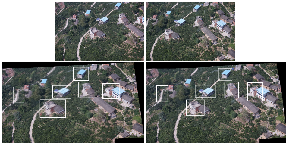
Figure 3. Mosaic results. The first row is the two images to be stitched together. The second row is two stitched images by global homography and local homography, respectively. White boxes highlight the ghostly parts.
