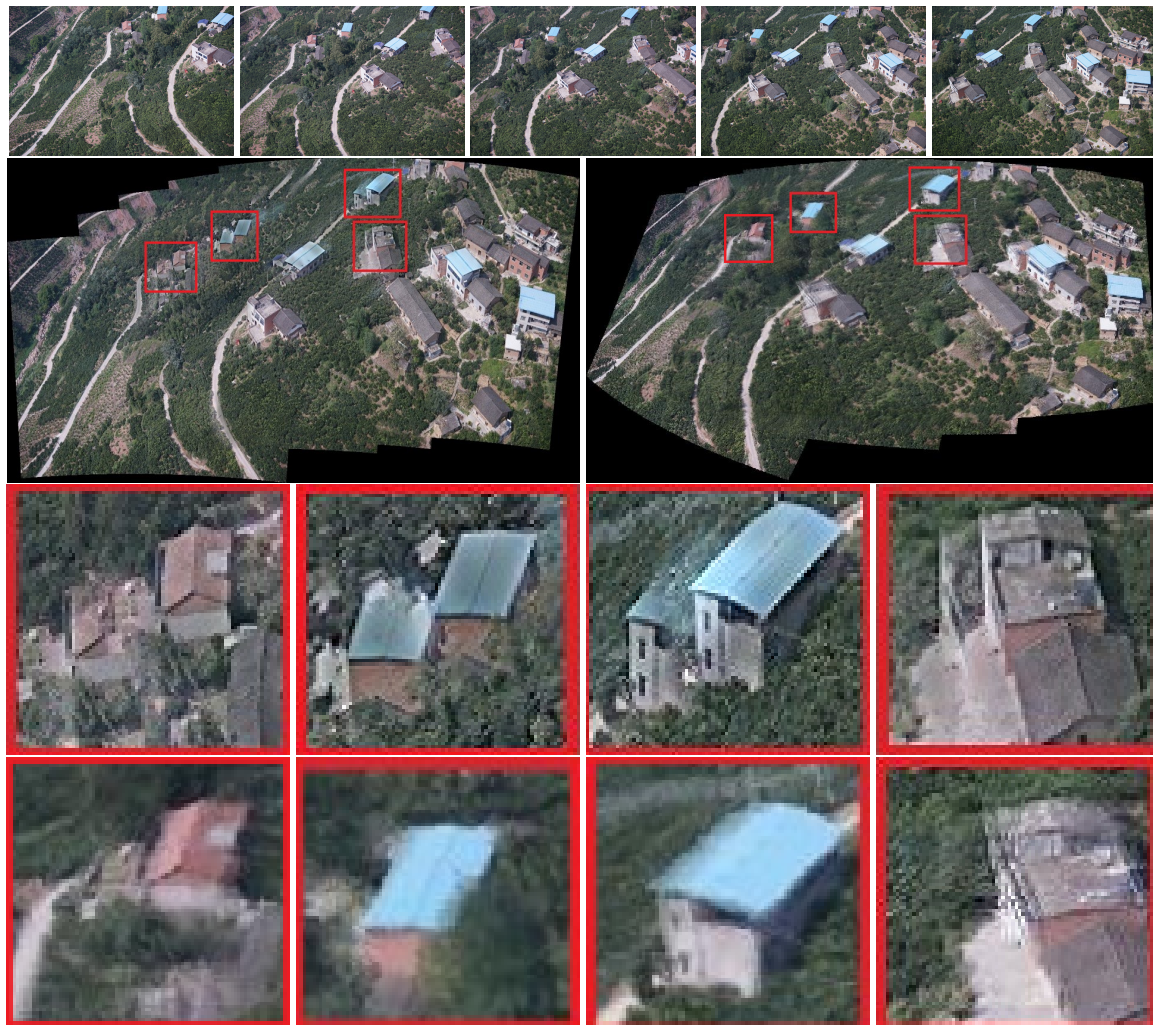
Figure 8. Experimental results of panoramic stitching. The first row is the image to be stitched together. The second row is the results of Autostitch and our method. Red boxes highlight the ghostly parts. The last two rows are the details of the red boxes.
