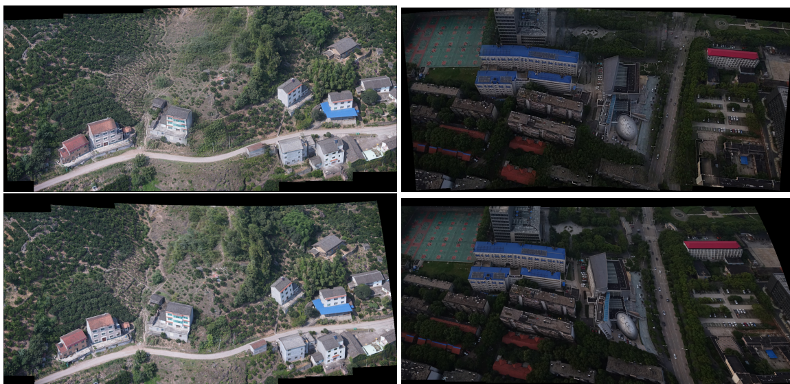
Figure 7. Experimental results of panoramic stitching. The source images are sequential images captured from left to right without nonrigid changes and parallax. The first row is the results of Autostitch. The second row is the results of our method.
