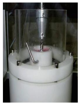
Fig. 2. The forces are applied in 45-degree angle over the crowns.
