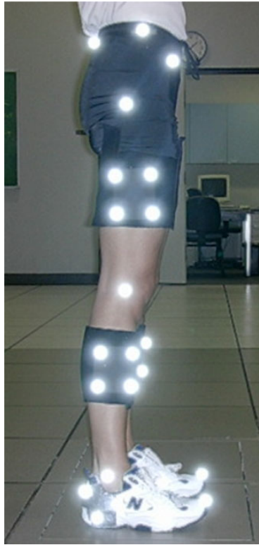
Figure 1. Lower extremity reflective marker placement.
