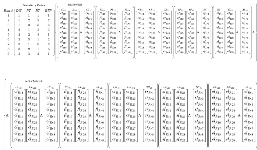
Fig. 5. A generalized L_9(3^4) OA dataset arrangement for the concurrent screening of the five sensory traits.
