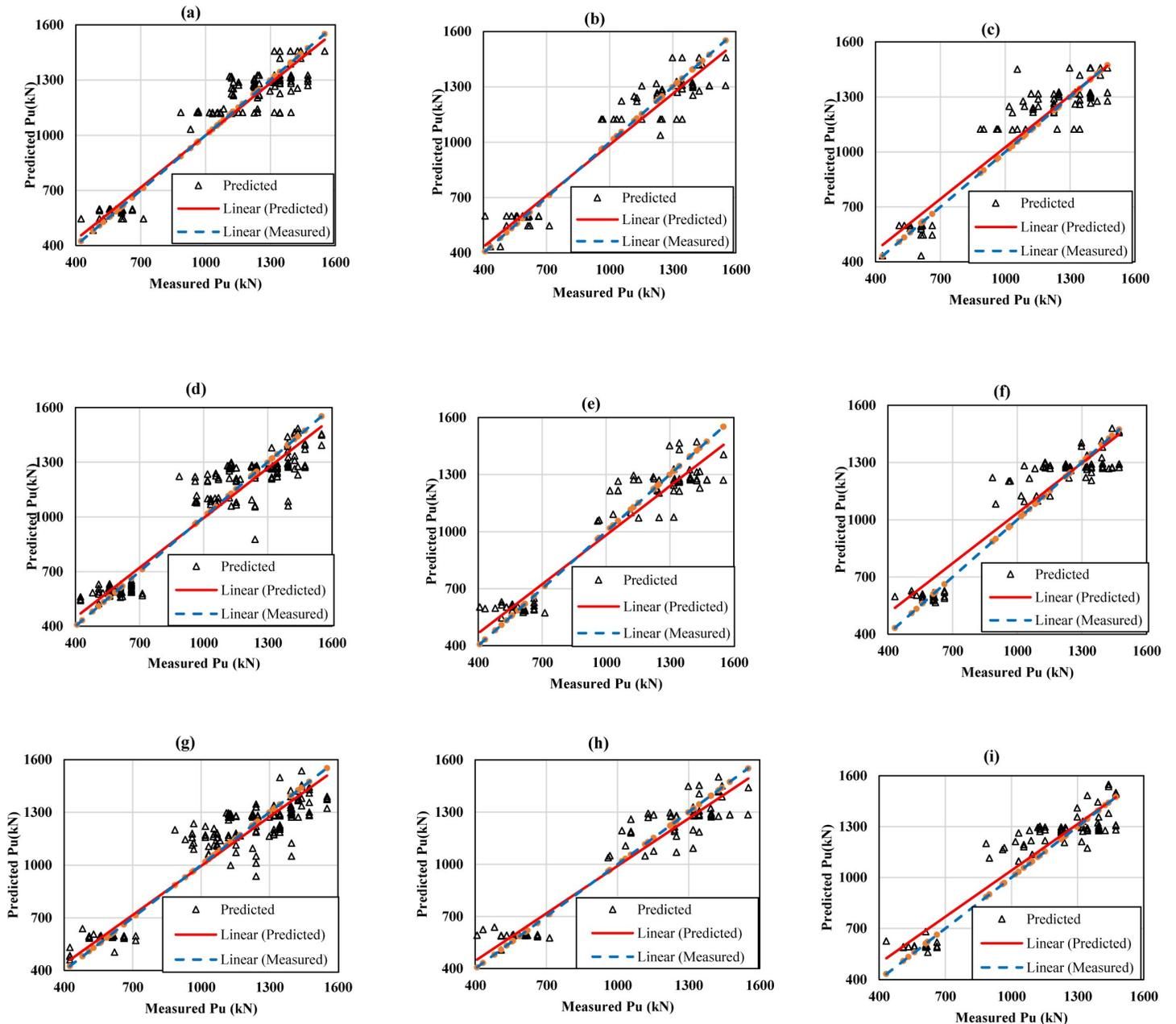
**Fig 10.** Measured and predicted values of axial bearing capacity of pile using the models: 4-input GA-DLNN model for training (a), validation (b), testing dataset (c); 10-input GA-DLNN model for training (d), validation (e), testing dataset (f); 4-input DLNN model for training (g), validation (h), testing dataset (i).
