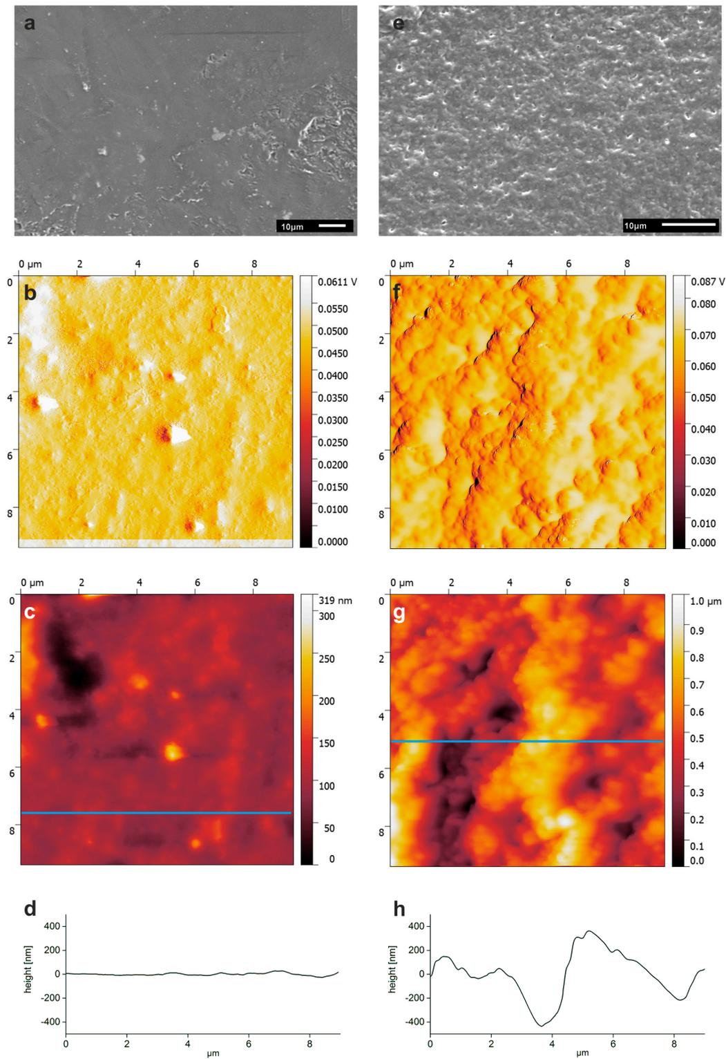
**Figure 3.** SEM and AFM data on as-printed (a–d) and NaOH-treated (e–h) PLA scaffolds. (a,e) SEM images; (b,f) AFM amplitude image; and (c,g) AFM topography image with corresponding height profiles. Blue lines in the images indicate position of the height profiles shown in (d,h).
