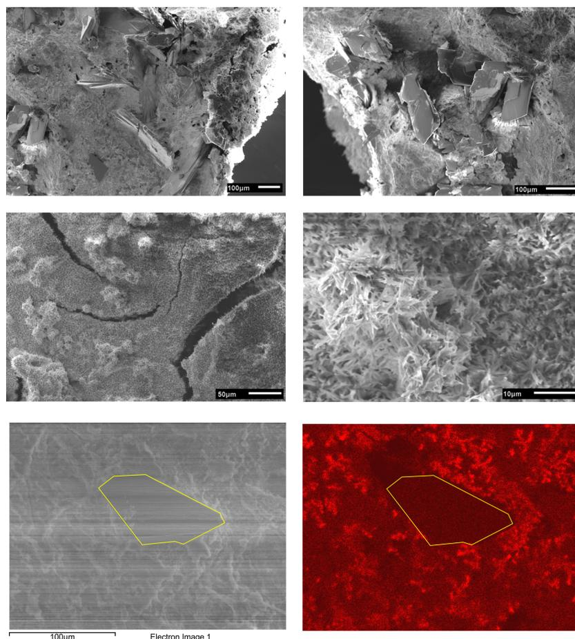
**Figure 9.** Representative SEM images of a chitosan/CP composite surface (sample C12). All images are from the same sample but taken at different locations and different magnifications to show the morphological and dimensional diversity. Bottom images show an Na elemental map in sample C12 and the corresponding SEM image. The plates are essentially sodium-free and the surrounding area shows a sodium content of ca. 5 atom %.
