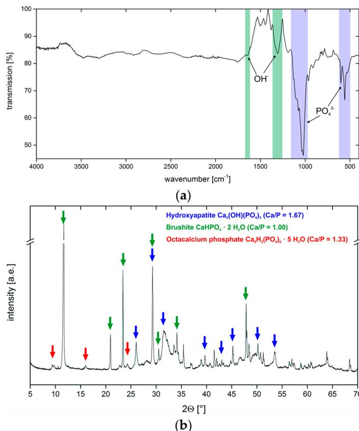
**Figure 10.** (a) IR spectrum obtained from sample C12. The other IR spectra are essentially identical with varying intensities of individual bands. (b) X-ray diffractogram of sample C20. The other diffractograms are essentially identical with varying intensities of individual reflections.
