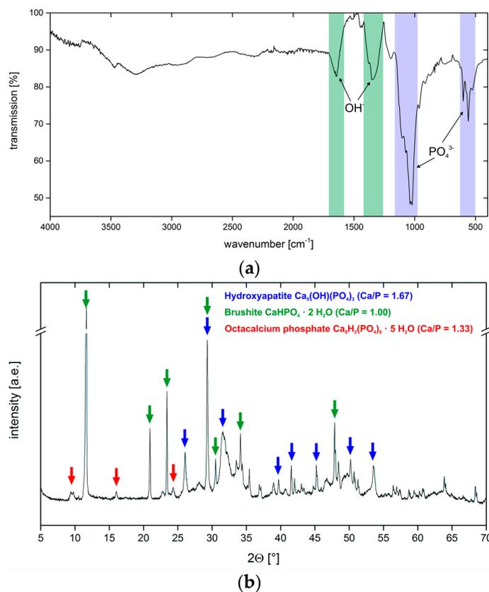
**Figure 7.** (a) Representative IR spectrum of the sample G01 (see Table 3 for sample designations). The other IR spectra are essentially identical with varying intensities of individual bands. (b) Representative XRD pattern of the sample G06. The other diffractograms are essentially identical with varying intensities of the individual reflections.
