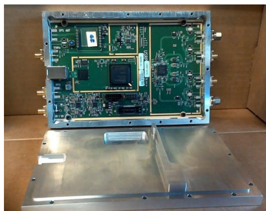
Figure 3. Photograph of the B210 USRP circuit board mounted inside its custom shielded housing and associated cover, which exhibits a central ridge that isolates RF fields from the digital portion of the circuitry.
