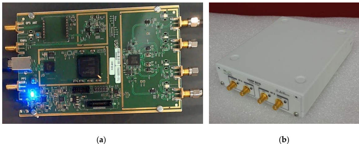
Figure 2. Photographs of the B210 USRP circuit board (a) without and (b) with a commercial cover.
