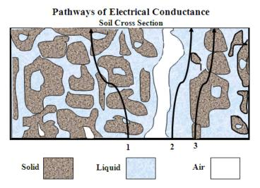
**Figure 1.** Three conductance pathways for the  $\sigma_h$  measurements, inspired by Wyllie and Southwick [11].
