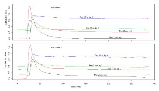
**Figure 3.** Bulk electrical conductivity ( $\sigma_b$ ) in the two soil columns for two irrigation events (N°.3 and N° 4) at two depths (21 cm and 35 cm). Series peaks are related to time irrigation.
