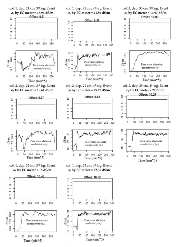
**Figure 6.** Estimation of the unobservable data ( $\varepsilon_{\sigma b=0}$  and  $\sigma_p$ ) by applying the time-varying dynamic linear model (DLM) and the Kalman filter on the data according to the soil column number (col.), depth (dep.), and irrigation event (irg. Event), the corresponding of  $\sigma_p$  by EC meter device is given for each estimated  $\sigma_p$ .
