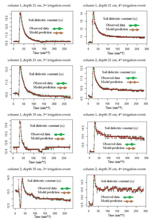
**Figure 5.** Observed and predicted soil relative dielectric permittivities according to the soil column number, depth, and irrigation event.
