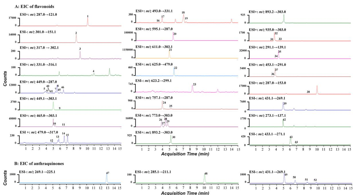
**Fig. 1.** Extracted ion chromatograms of 52 compounds identified in Tartary buckwheat sprouts, including 46 flavonoids (A) and 6 anthraquinones (B). These compounds were all studied in the positive ion mode (ESI +), with the exception of compounds 2, 23, 43, 44, and 47–52. Compound number is in agreement with those in [Table 1](#).
