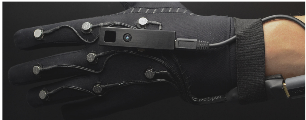
Figure A2. The matrix of 3 \times 3 LRA vibration motors forming the haptic interface of the prototypes—in this case an early prototype is shown.
