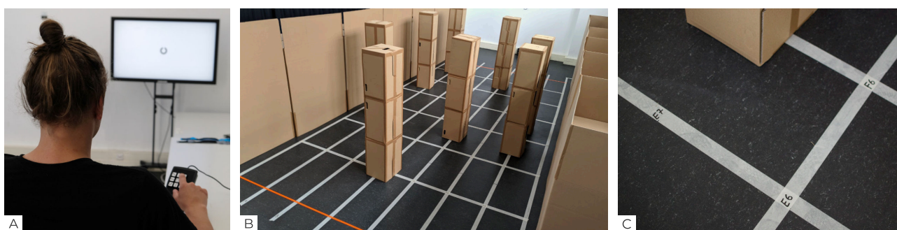
Figure 2. (A) Carrying out the "FrACT" Landolt visual acuity test with screen and tactile input device (lower right corner). (B) The obstacle course in the study room. (C) Close up of the grid system used for quick rebuilding of the layouts.
