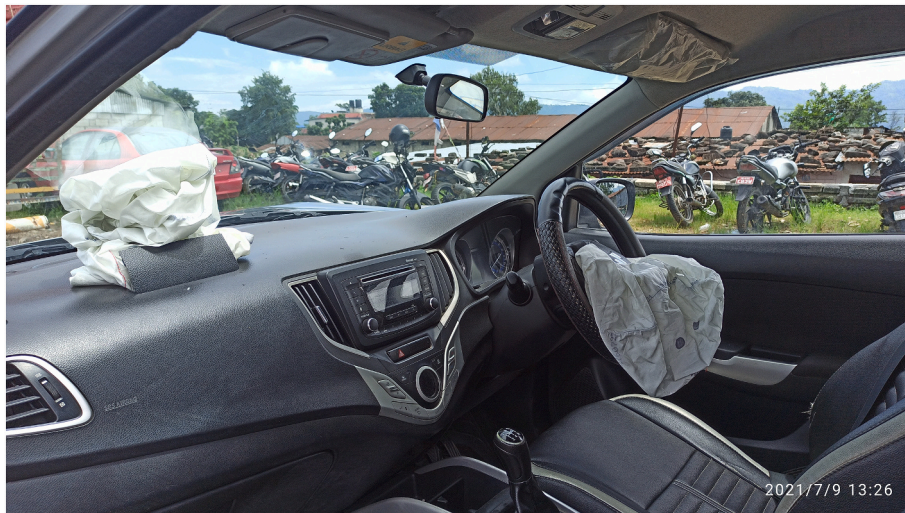
Fig. 2. Figure 2 shows the deployment of air bags at both the sides (Driver side and passenger side).
