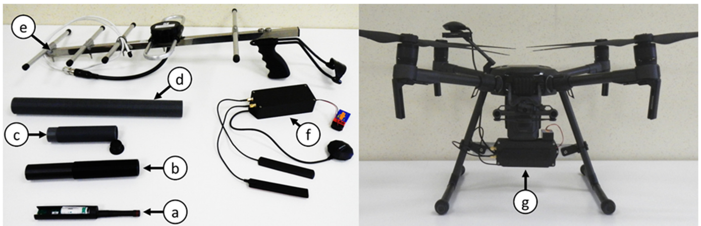
Figure 4. (a) Kinematic Logger, battery, and 433 MHz antenna installed in a 3D printed sleeve, (b) threaded waterproof housing for the Kinematic Logger, (c) threaded end plugs to span the distance between the Kinematic Logger and the surface of the stone, (d) threaded sleeve that is glued into the stone, (e) directional Yagi antenna with handle and wrist support for Kinematic Logger recovery missions, (f) relay unit with antennas and 9 V battery, (g) relay unit installed on a DJI M210 UAV.
