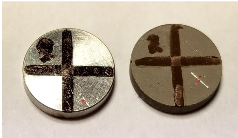
Figure 3. Titanium discs used, the site of irradiation marked with a red circle; machined surface to the left and sandblasted and acid-etched to the right.
