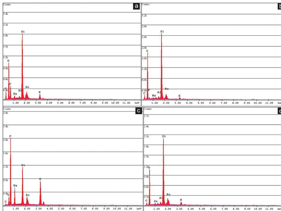
**Figure 4:** Elemental analysis of the surface of rods in the four groups by EDS: (a) group 1; (b) group 2; (c) group 3; and (d) group 4
