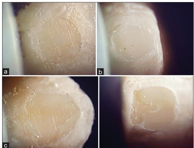
Figure 2: Modes of failure. (a) Adhesive; (b) cohesive; and (c) mixed
