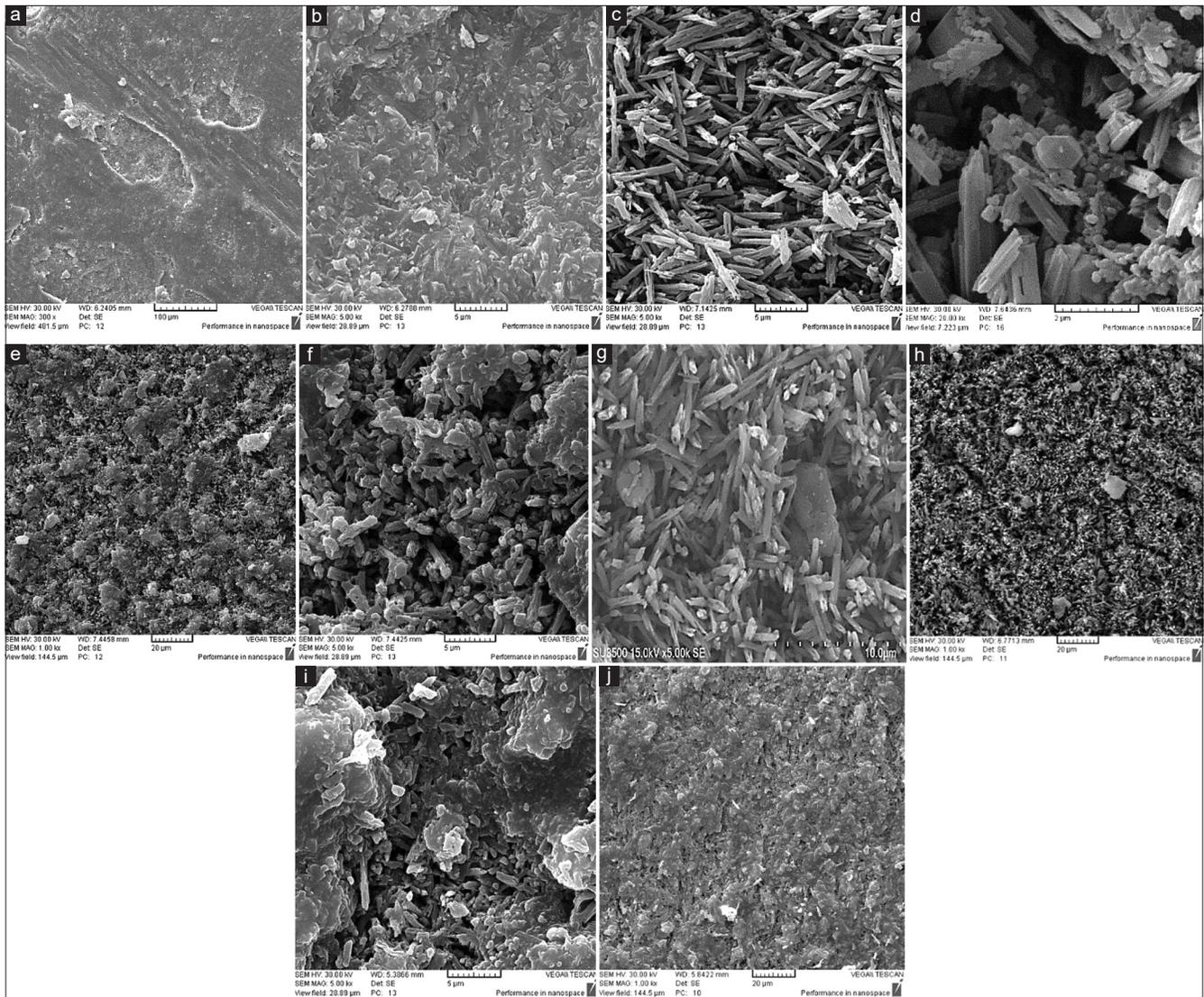
**Figure 3:** SEM micrographs of the cross-sectional areas of rods in different groups; (a and b) no surface treatment; (c and d) 5% HF acid for 20 seconds; (e and f) 5% HF acid + AI with a microbrush each for 20 seconds; (g and h) 5% HF acid for 20 seconds and 32% PA for 40 seconds; (i and j) 5% HF acid for 20 seconds and 32% PA for 40 seconds + AI with a microbrush for 20 seconds ( $\times 1000$  and  $\times 5000$  magnifications)
