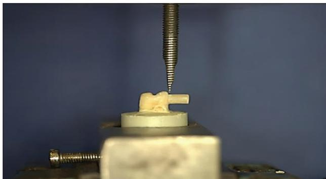
Figure 1: Load application in a universal testing machine
