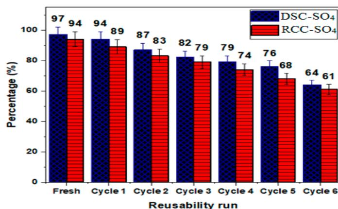
**Figure 5.** The reusability of the mesoporous DSC-SO<sub>4</sub> and RCC-SO<sub>4</sub> catalysts for six reaction runs at optimum reaction conditions.
