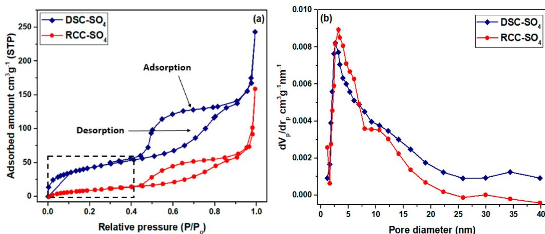
**Figure 1.** (a) N<sub>2</sub> adsorption–desorption isotherms and (b) pore size distribution profiles of dual-stage char-derived (DSC)-SO<sub>4</sub> and rising co-current char-derived (RCC)-SO<sub>4</sub> catalysts.
