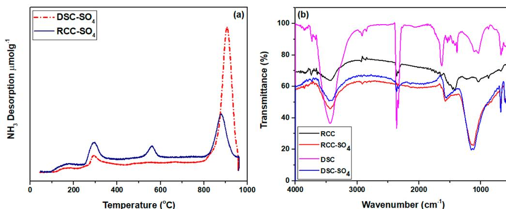
**Figure 2.** (a)  $\text{NH}_3$ -TPD profiles of the synthesized mesoporous DSC- $\text{SO}_4$  and RCC- $\text{SO}_4$  catalysts and (b) FT-IR spectra of DSC, DSC- $\text{SO}_4$ , RCC, and RCC- $\text{SO}_4$  samples.
