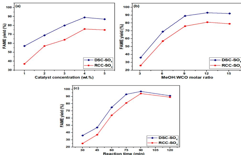
**Figure 4.** (a) Influence of catalyst concentration on fatty acid methyl esters (FAME) conversion; (b) influence of MeOH/waste cooking oil (WCO) molar ratio on FAME conversion; (c) influence of reaction time on FAME conversion.
