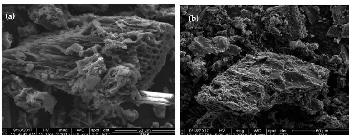
**Figure 3.** FE-SEM images of the mesoporous (a) DSC- $\text{SO}_4$  and (b) RCC- $\text{SO}_4$  catalysts.
