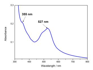
Figure 6. UV–Vis absorption spectrum of a 20/80 MPTMS/TEOS films after immobilizing [Fe(bpy)<sub>3</sub>]<sup>2+</sup>.
