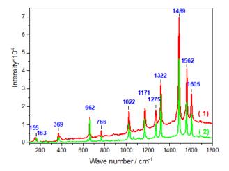
**Figure 4.** Comparison of the Raman spectra of  $[Fe(bpy)_3]^{2+}SO_3^-@SiO_2$  film (red, 1) and the Raman spectra of  $[Fe(bpy)_3]SO_4 \bullet 7.5H_2O$  microcrystalline powder (green, 2).
