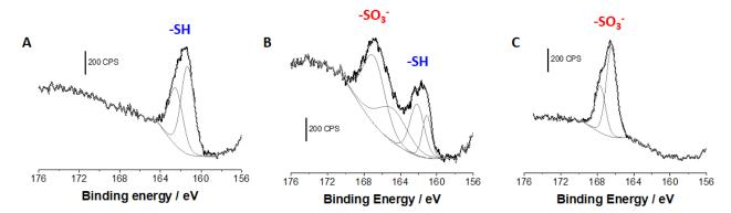
**Figure 2.** S2p core level spectra of a mercaptopropyl-functionalized mesoporous silica film (obtained by EASA from a sol prepared from 20/80 MPTMS:TEOS), respectively, recorded before (**A**), after  $10 \text{ min } (\mathbf{B})$ , and after  $30 \text{ min } (\mathbf{C})$  of chemical oxidation with hydrogen peroxide (30%) in  $0.1 \text{ M H}_2\text{SO}_4$ .
