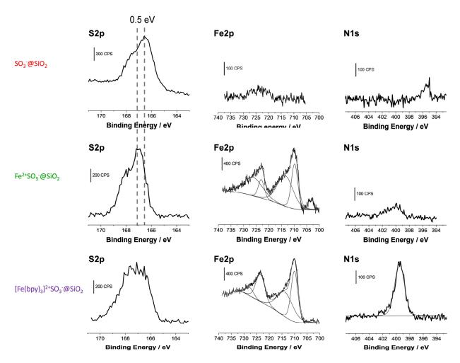
**Figure 3.** S2p (left), Fe2p (center) and N1s (right) core level spectra recorded for 20/80 films, respectively, functionalized with sulfonate groups ( $SO_3^-@SiO_2$ , top), after complexation with iron (II) (Fe<sup>2+</sup>SO<sub>3</sub><sup>-</sup>@SiO<sub>2</sub>, middle) and after Fe<sup>2+</sup> complexation and bipyridine displacement of aquo ligands ([Fe(bpy)<sub>3</sub>]<sup>2+</sup>SO<sub>3</sub><sup>-</sup>@SiO<sub>2</sub>, bottom).
