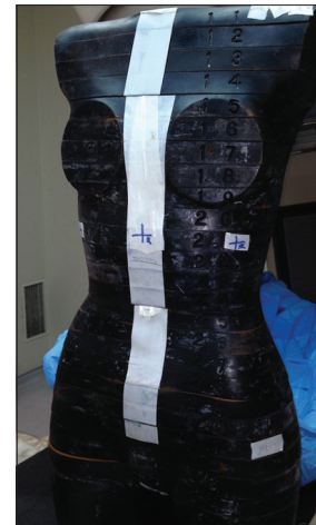
Figure 1: Alderson female RANDO phantom, which was used in this study to simulate a breast cancer patient at 8 weeks of pregnancy who has no abdominal enlargement
