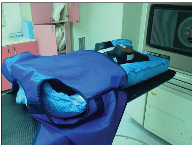
Figure 4: The placement of lead apron over the phantom. The apron covered the abdominal region of the phantom loosely, to ensure the comfort of the simulated pregnant patient
