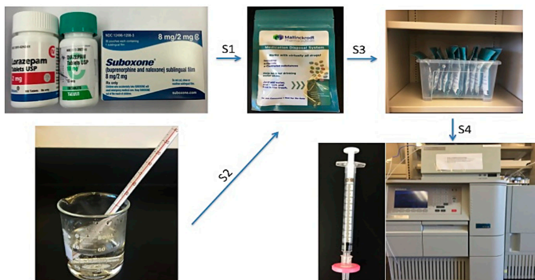
Figure 1. Schematic representation of deactivation study of psychoactive medications. S1: Medications were added to the deactivation pouches; S2: 50 mL warm tap water was added to each pouch; S3: Pouches were stored upright and undisturbed at room temperature; S4: Samples were collected at different time points and analyzed by HPLC.
