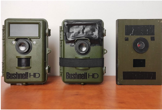
FIGURE 1 Bushnell Natureview ® HD trail camera used for nest box monitoring. From the left: trail camera with 250 mm lens without custom modifications, trail camera with IR LED lights covered with a black plastic wrap and PIR motion sensor covered with opaque rubber band, dummy trail camera
