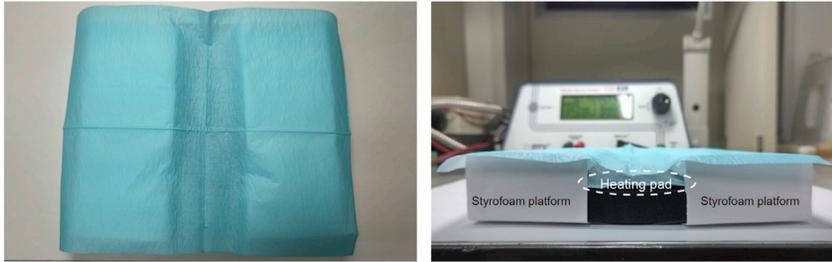
**Figure 4. Operating table for *in utero* electroporation**
