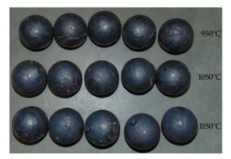
Figure 5. Shape of balls formed from 40 mm-diameter billet of varying initial temperatures.
