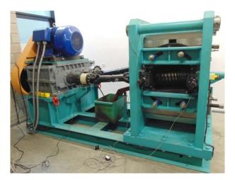
Figure 2. Helical rolling mill used in the experimental tests.
