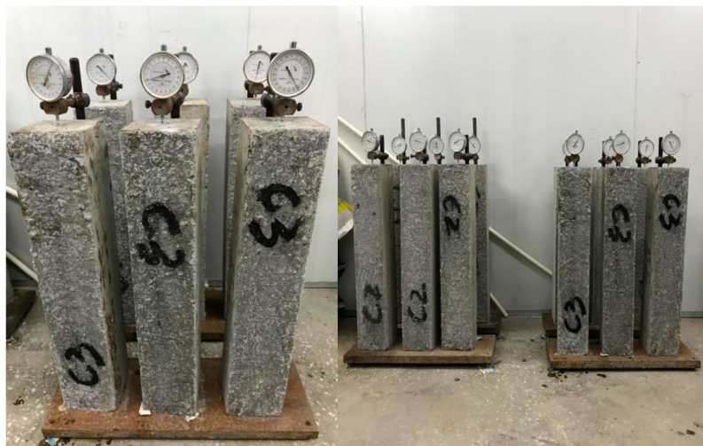
Figure 5. Drying shrinkage test of GO concrete.
