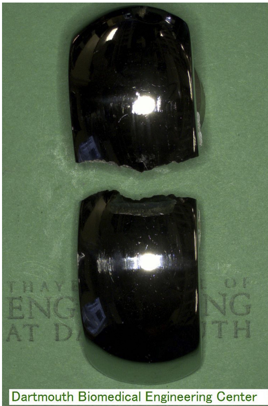
Figure 5. Explanted Vanguard femoral UKA component.
