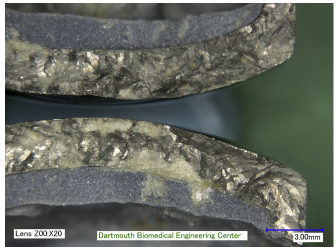
Figure 6. Close-up of fracture through femoral UKA component with evidence of fatigue striations.
