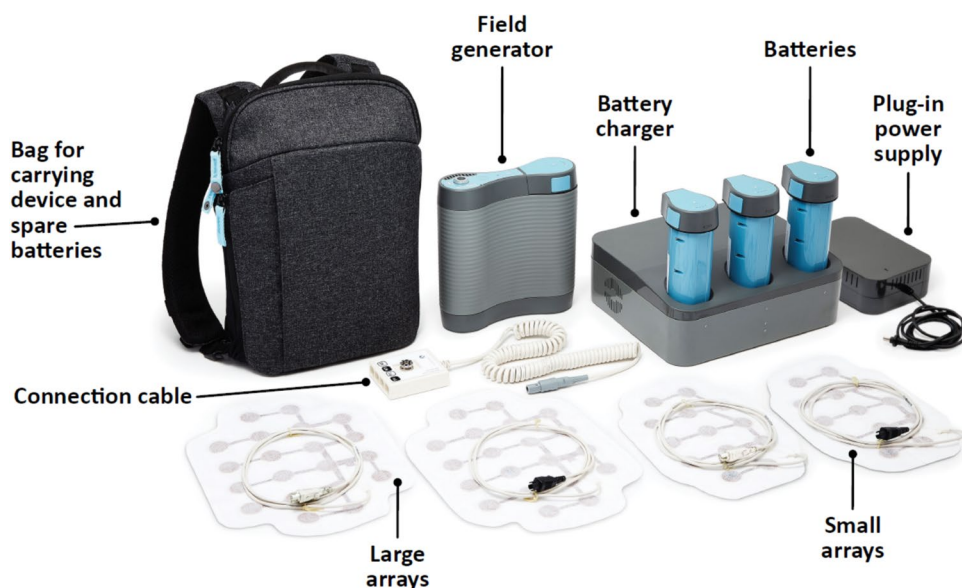
Fig. 1 The NovoTTF™– 200 T system is comprised of an electric field generator and new generation arrays. It is the first device indicated to be used in conjunction with standard chemotherapy to treat patients with unresectable pleural mesothelioma, US Food and Drug Administration approval date: May 23, 2019 [34].
