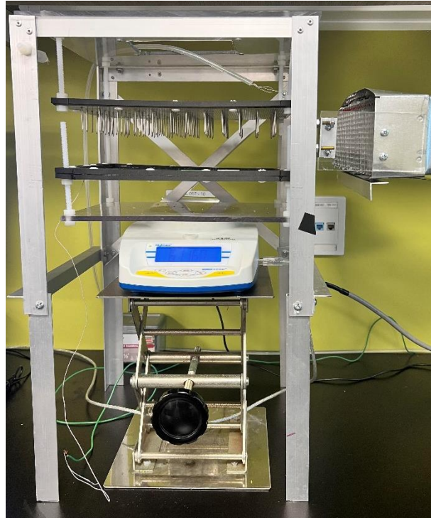
Figure 1. Electrode arrangement in EHD dryer.
