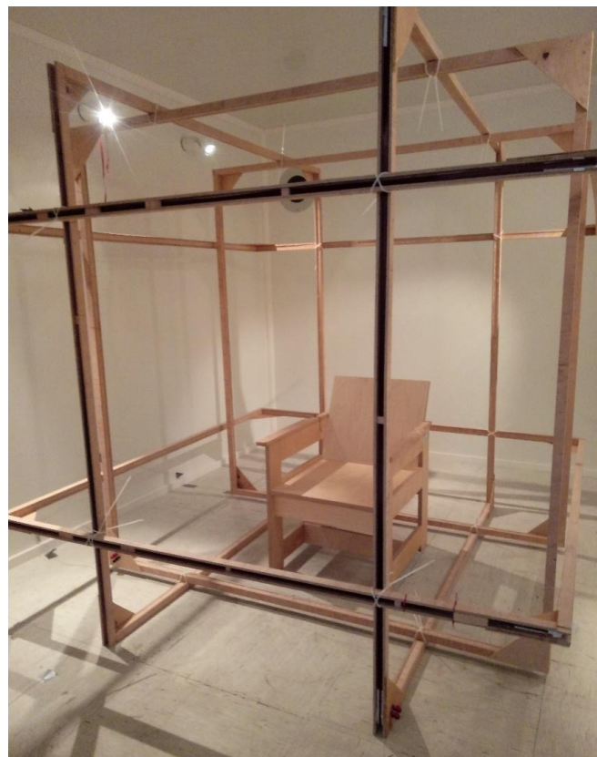
Figure 3. Wooden Helmholtz coils setup installed in a two-layer magnetically shielded room (Vacoshield Advanced, Vacuumschmelze GmbH & Co. KG, Hanau, Germany) at Warsaw University of Technology, Faculty of Mechatronics.
