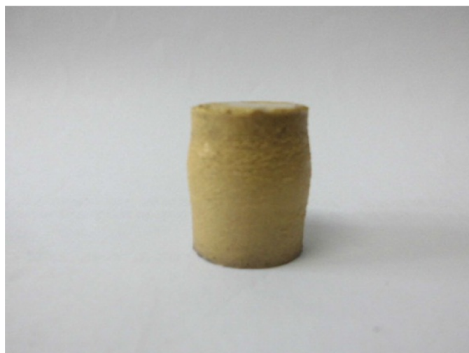
Figure 15. Compressive strength test deformed sample and test results.
