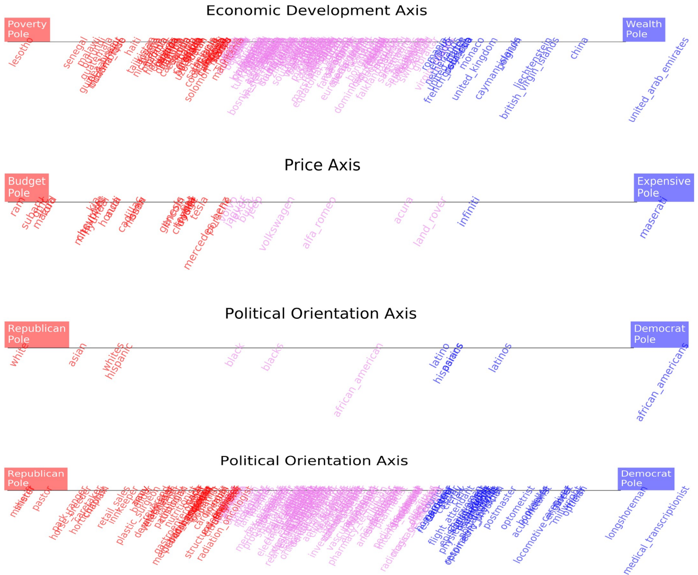
Fig 11. Cultural axes do not need to be circumscribed to clear cut concepts such as gender. Arbitrary axes describing economic development, socioeconomic status or political orientation can be created. Projecting relevant word vectors onto those axes reveals the associations contained in the corpus (Google News in the Figure) on which the word embedding model (word2vec) was trained.
