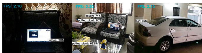
Fig. 17. Images of real-time detected objects with non-solid backgrounds and different lighting conditions by Raspberry Pi.
