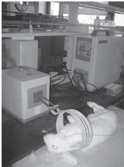
Figure 3. Experimental apparatus of the magnetic hyperthermia system (MHS).
