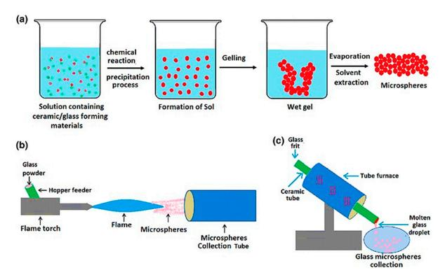
**Figure 6.** Illustration of glass microsphere production by the (a) sol-gel, (b) flame spheroidization, and (c) furnace methods. Figure retrieved from (Hossain et al. 2015) [49].
