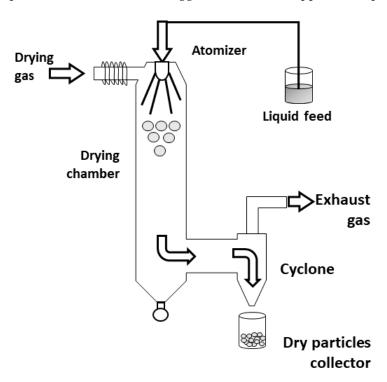
Figure 8. Schematic of spray-drying process. Figure adapted with permission from Sosnik et al. [64].
