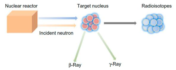
**Figure 3.** Schematic representation of nuclear reaction between a target nucleus and an incident neutron, leading to the formation of a radioisotope and the emission of beta and/or gamma rays. Figure reproduced from Deliberato Aspasio et al. [27].
