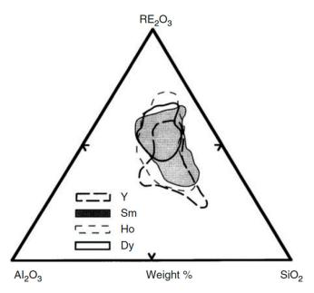
**Figure 4.** Compositional ternary diagram showing the glass formation range for REAS compositions that melt below 1600 °C. Yttrium, while not being rigorously a rare earth element, is comprised in the diagram because it has similar properties to those of rare earths [12].
