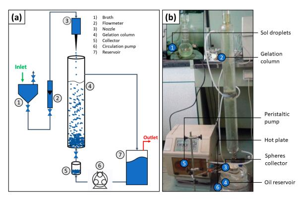
**Figure 7.** (a) Schematic of a generic internal gelation apparatus and (b) picture of a typical experimental setup. Figures (b) adapted with permission from Poorbaygi et al. [59].
