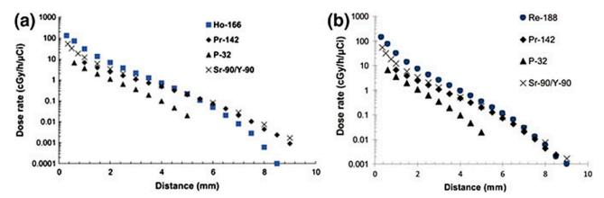
**Figure 9.** Comparison of the dose rate vs. distance for different glasses containing beta emitters. Figure adapted from Hosseini et al. [76] (a) and Khorshidi et al. [77] (b).
