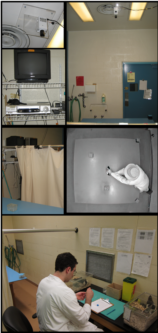
Figure 4: Photographs of experimental setup in studies using an animal model of OCD. Top row shows photographs of the ceiling-mounted video camera focused on the open field, fluorescent lighting illuminating the testing room, and a VCR-monitor station standing on shelves attached to the wall. Middle row, left photo, shows the partially drawn curtain between the open field and the VCR-monitor station; right photo is a screen capture image from a video file showing the experimenter placing a rat onto the open field. Bottom photo is of the workbench located between the 2 curtains separating the open fields. On the workbench are 2 home cages with a rat inside. Experimenter prepared syringes with the drug solution, administered the drug treatment, and placed the rat on the open field. Experimenter was present in the testing room throughout the trial but was hidden behind a curtain from the animal's sight. Experimenter observed activity of the rat on a TV monitor and retrieved the rat if it fell or jumped off the arena. The rat was generally placed back at the spot from which it left the arena. Montage is of photos taken at different times, from 2004 to 2010.
