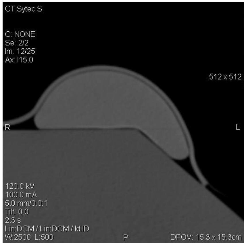
FIG. 3. Slice of the CT study performed using the breast implant phantom covered with the TiLOOP Bra mesh and 5 mm bolus. No metallic artifacts are observed.
