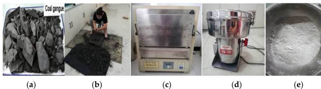
Figure 1. Flow diagram of preparation of UCGP. (a) raw coal gangue, (b) manual smash, (c) calcined 2 h, (d) crushed it, (e) UCGP.
