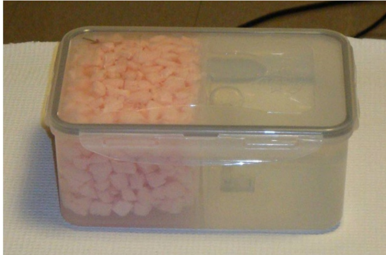
FIG. 2. The phantom used for our studies. It consists of a watertight plastic box with two sections designed to represent lung and liver.
