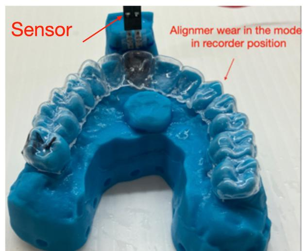
Figure 3 Illustration of measuring the corrective force of the invisible aligner.
