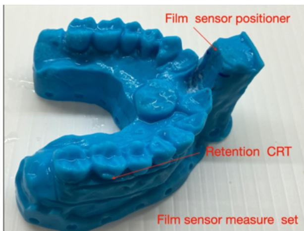
Figure 2 Measurement model ( $M_t$ ) used for measuring corrective force.
