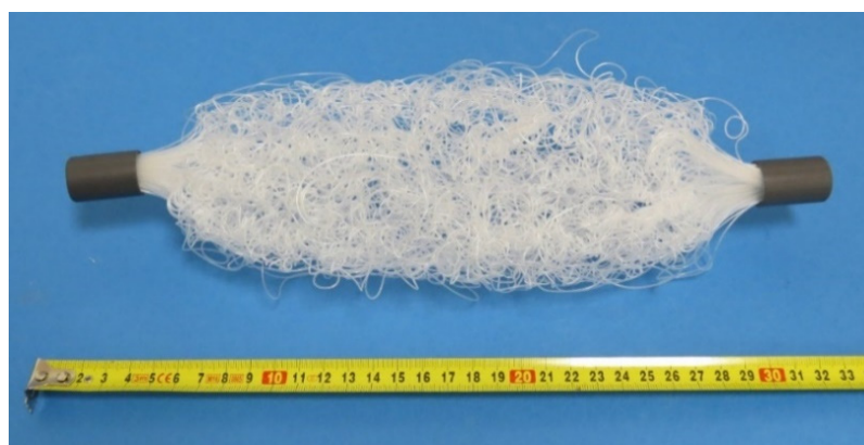
Figure 2. A condenser made of non-porous polypropylene hollow fibers.
