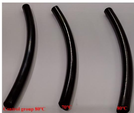
Figure 2. Surface photos of EPDM rubber before and after the test.
