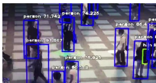
Figure 7. Automatic determination of the number of people using image-recognition technology.
