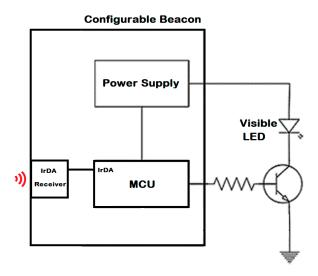
Figure 4. The beacon block diagram.
