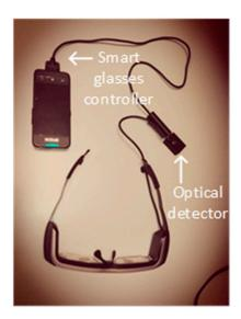
Figure 16. EPSON BT-200 smart glasses, model H560A, with receiver connected to the jack port.
