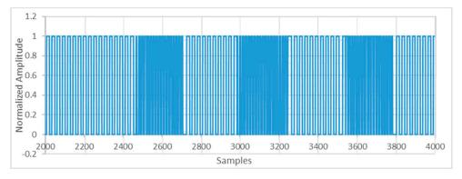
Figure 10. Reshaped signal through simple threshold algorithm.
