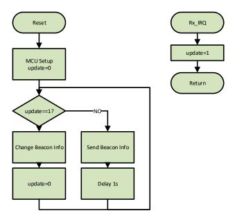
Figure 2. Flowchart of the beacon firmware.
