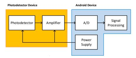
Figure 5. Block diagram of the receiver module.
