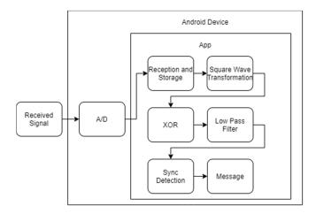
Figure 8. Application block diagram.
