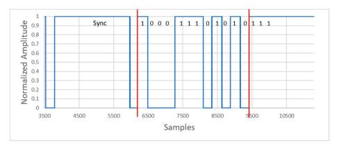
Figure 15. Synchronization and message bits after processing.
