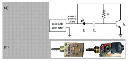
Figure 6. Receiver module (a) schematic and (b) PCB-Mount circuit.
