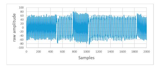
Figure 9. Signal recorded through the audio jack.
