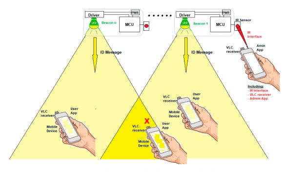
Figure 1. VLC beacon system based on proximity algorithm.
