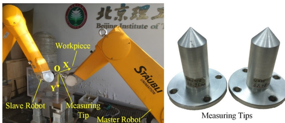
Figure 5. A typical calibration process of workpiece frame.
