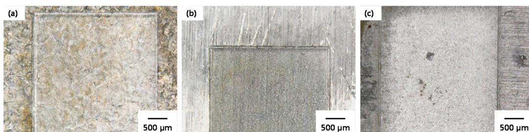
Figure 11. Micro-impresions produced under the optimized laser parameters on; (a) TiA, (b) NiA, (c) AlA.
