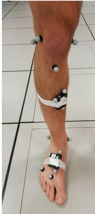
Figure 2. Illustration of the criterion-related validation set-up: Anatomical (applied to bony landmarks) and technical (applied to sensors boxes) markers, as well as the two IMUs, affixed on the right foot (along the second metatarsal) and leg (medial upper shank) of the participant, are represented. Among the anatomical markers, only the second and fifth metatarsal, and calcaneal tuberosity markers were used for this study. No marker was present for the construct validation study.
