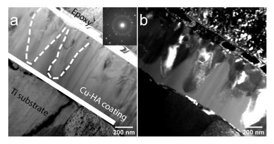
**Figure 6.** TEM image of the cross-section of Cu-HA coating on Ti after HT at 450 °C BF, the inset shows the corresponding electron diffraction pattern (**a**) and DF (**b**).
