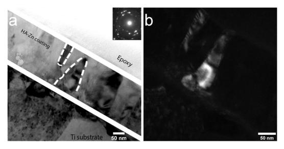
**Figure 12.** TEM image of the cross-section of Zn-HA coating on Ti deposited at the substrate temperature of 400 °C BF, the inset shows the corresponding electron diffraction pattern (**a**) and DF (**b**).
