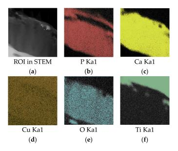
**Figure 8.** An energy dispersive X-ray (EDX) element mapping of the Cu-HA and Ti substrate in TEM lamella. (a) ROI in STEM; (b) P Ka1; (c) Ca Ka1; (d) Cu Ka1; (e) O Ka1; (f) Ti Ka1.
