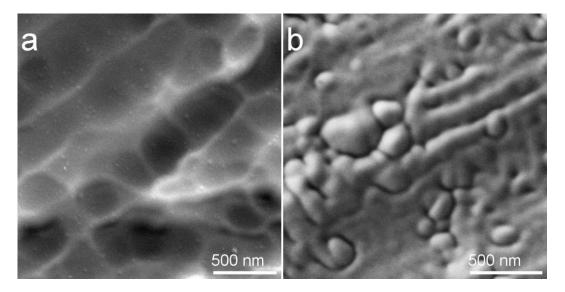
Figure 3. As-deposited Cu-HA coating on Mg0.8Ca (a) and on Ti substrate (b).
