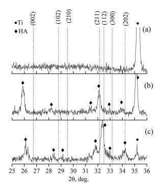
**Figure 2.** X-ray profiles of Cu-HA coating on Ti as-deposited (**a**), Cu-HA coating on Ti after annealing at 450 °C for 3 h (**b**) and Cu-HA coating on Ti after annealing at 700 °C for 3 h (**c**).
