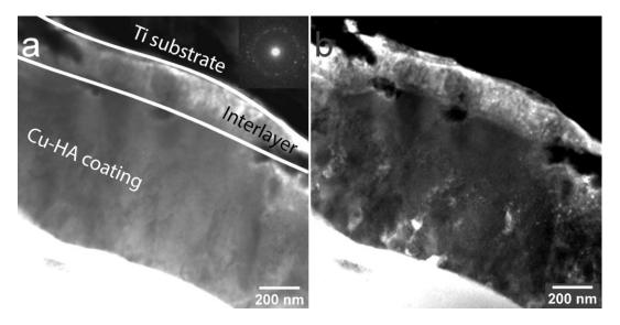
**Figure 7.** TEM image of the cross-section of Cu-HA coating on Ti after HT at 700 °C BF, the inset shows the corresponding electron diffraction pattern (**a**) and DF (**b**).
