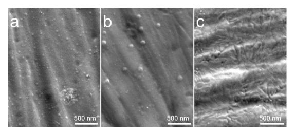
**Figure 11.** SEM images of Zn-HA coatings deposited at in situ substrate temperature 100 °C (**a**), 300 °C (**b**), and 400 °C (**c**).
