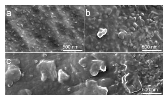
**Figure 4.** Scanning electron microscope (SEM) image of the Cu-HA coating on Mg0.8Ca alloy after HT at 450 °C showing fine crystallites (**a**) Cu-HA coating on Ti after HT at 700 °C showing the same type of crystallites of increased size(**b**) and Cu-HA coating on Ti after HT at 700 °C showing agglomerates of crystallites (**c**).
