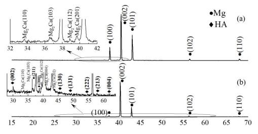
**Figure 1.** X-ray profiles of as-deposited Cu-hydroxyapatites (HA) coating on Mg0.8Ca (**a**) and Cu-HA coating on Mg0.8Ca after heat treatment (HT) at 450 °C for 3 h (**b**).
