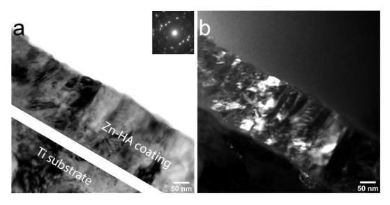
**Figure 13.** TEM image of the cross-section of Zn-HA coating on Ti deposited at the substrate temperature of 400 °C BF, the inset shows the corresponding electron diffraction pattern (**a**) and DF (**b**).
