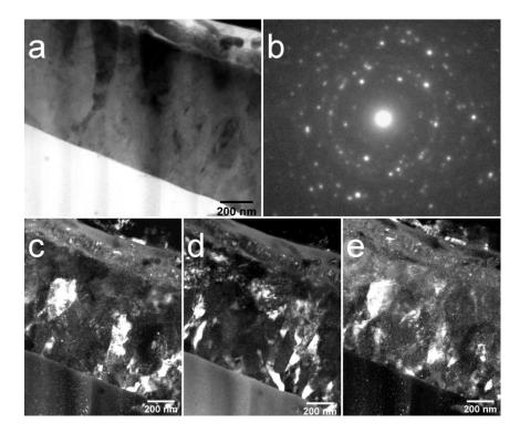
**Figure 9.** TEM image of the cross-section of Cu-HA coating on Ti after HT at 750 °C BF image (**a**), selected area electron diffraction (SAED) obtained from the coating region (**b**), DF in reflex (002) (**c**), DF in reflex (112) (**d**), and DF in reflex (213) (**e**).
