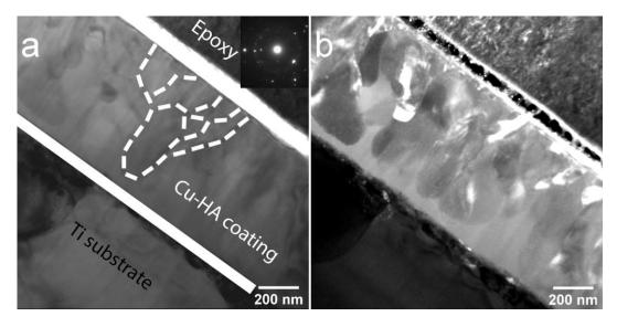
**Figure 5.** Transmission electron microscope (TEM) image of the cross-section of Cu-HA coating on Ti after HT at 450 °C bright field (BF), the inset shows the corresponding electron diffraction pattern (**a**) and dark field (DF) (**b**).
