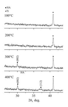
**Figure 10.** XRD profiles of Zn-HA coatings deposited at in situ substrate temperature 100 °C, 200 °C, 300 °C, and 400 °C.
