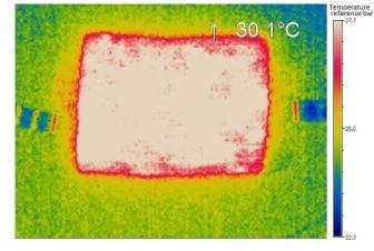
(b) Thermal image of rib knitted structure
