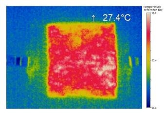
Figure 5. Thermal images for (a) plain; (b) rib and (c) interlock structures at 3 V.
