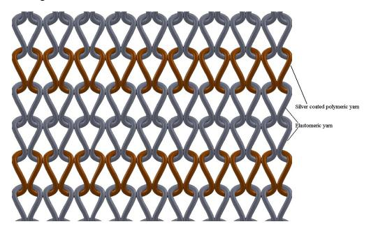
Due to the stretched elastomeric yarn, the silver yarn loops are pressed together at their sinker loops. The result would be that no electrical current flows in the heads of the knitted loop while the current only flows through the sinker loops. Using the simple knitted loop geometry put forward by P. Popper [31], the yarn geometry at the junction can be given by Figure 2.
