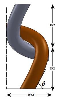
Figure 2. A binding point at the sinker loop of the knitted structure.
