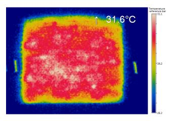
(c) Thermal image of interlock knitted structure
